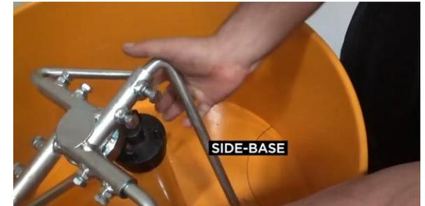
To mount the side-base arm lift up the cross joint.
