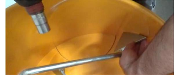
When the blade is 1-3 mm from the drum edge, fasten the bolts.
