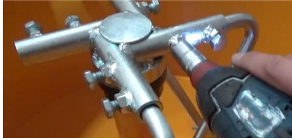
When the blade sits correctly, fasten the bolts - with spanner 16.
