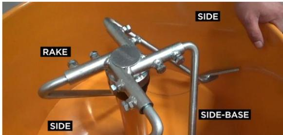
If you are changing all the arms, start with mounting the rake. Then mount a side arm on each side of the rake.
